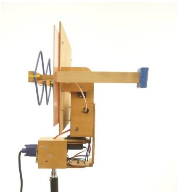
Figure 12 Elevation servo backward position
