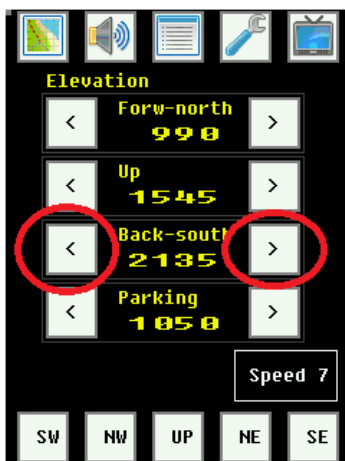
Figure 13 Adjust elevation backward position
