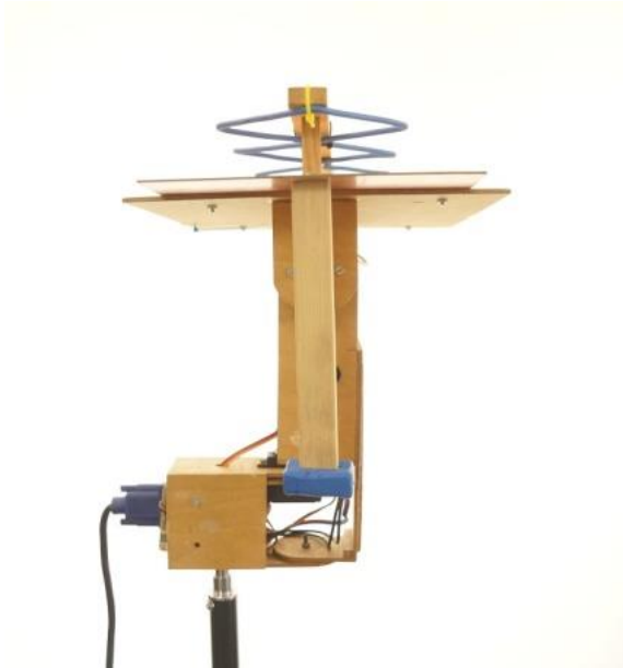
Figure 14 Elevation servo in center (up) position
