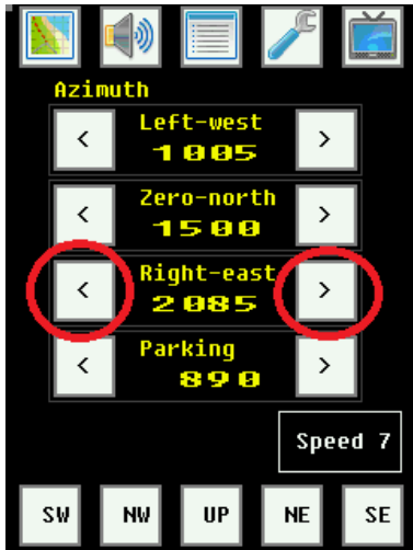
Figure 7 Adjust azimuth servo 90 deg CW position
