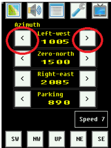
Figure 5 Adjust azimuth servo 90 deg CCW position
