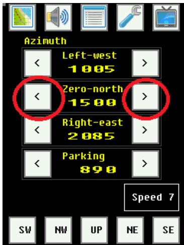
Figure 9 Azimuth servo zero adjustment
